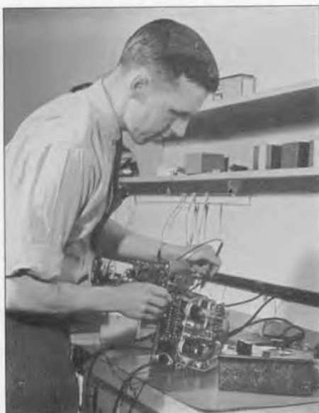
FIGURE 10. C. A. Woodward, of the Measurement Group, with the preliminary model of a high-frequency voltmeter.
