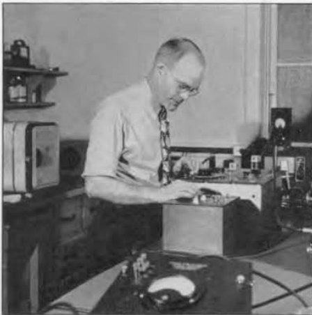
FIGURE 17. D. H. Chute, in charge of the measurements room, balances a precision capacitance bridge.
