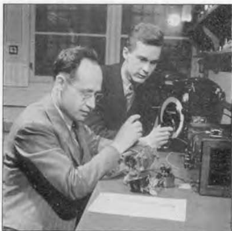
FIGURE 14. E. E. Gross (left) and W. R. Thurston, of the High-Frequency Group, working on a u-h-f oscillator of the coaxial butterfly type.
