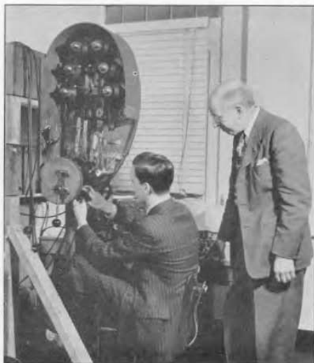
FIGURE 12. R. F. Field (right) and D. A. Powers, with a machine for winding polystyrene capacitors, a new type developed under Mr. Field's supervision.
